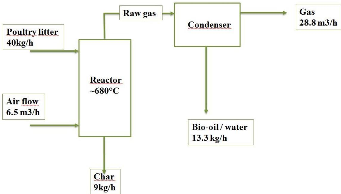
Figure 1: Schematic diagram of the on farm up-draft gasifier
