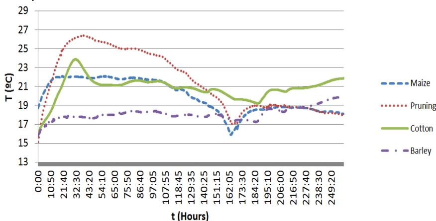
**Fig 1.** Temperature evolution from the composting simulator test of SPS with several bulking agents.
