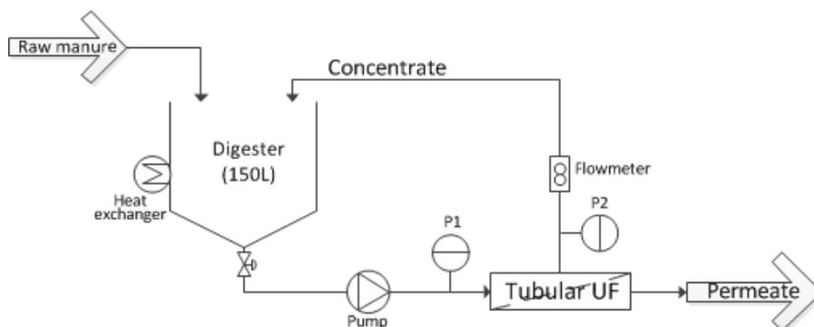
The UF experiments were performed by BioScan A/S using polyethersulphone (PES) tubular membranes (40kDa). The digestate feed was produced in a pilot scale plant (Figure 2).
