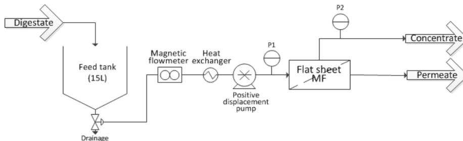
M10 laboratory plant (Figure 1). The feed stream was the centrifuged digestate liquid fraction from Fangel Biogas (Denmark).
