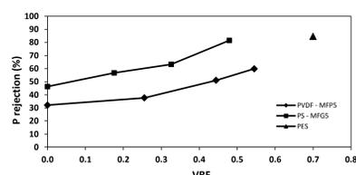
Figure 8: Phosphorus rejection for the ultimate concentrate obtained during concentration tests (shown in Figure 6-7)
