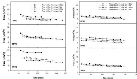
Figure 4: Filtration tests using PVDF membranes (left) and PS membrane (right)
