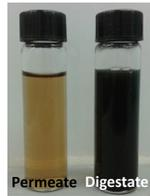
Figure 1: Permeate after filtration (left), digestate liquid fraction (right)
