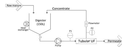
Figure 3: UF pilot plant (Bioscan A/S)
