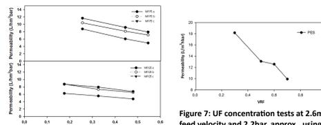
Figure 6: MF concentration tests at 1.4m/s feed velocity and 1bar, using MFP5 (triplicate) and MFG5 (triplicate)
