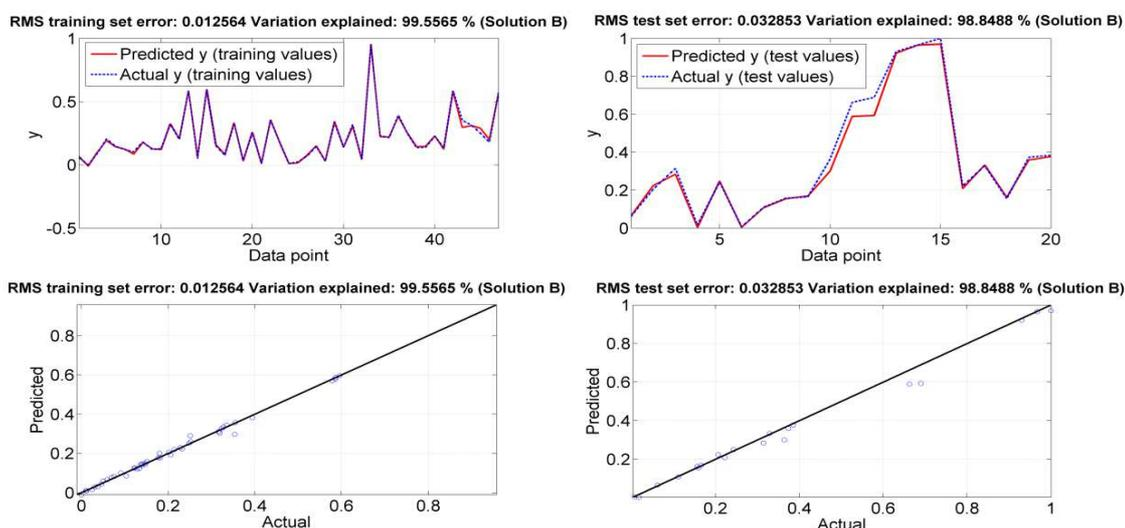
Figure 1. Prediction results with MGGP (Solution B) on the training and the testing dataset for Syngas yield production
