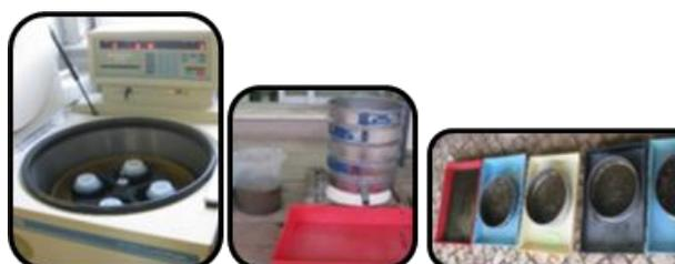
Fig. 1 Laboratory centrifuge and five sieves used on the separations
